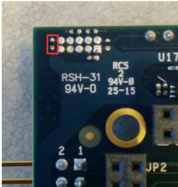
Figure 5-1: Location of R1 highlighted on bottom side of Apollo base board, next to J8
