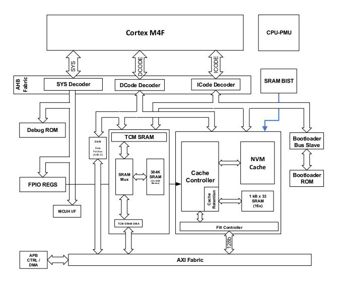
Figure 3. Apollo4 Blue Lite SoC Core Block Diagram
