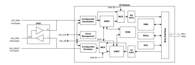
Figure 46. I<sup>2</sup>S Block Diagram
