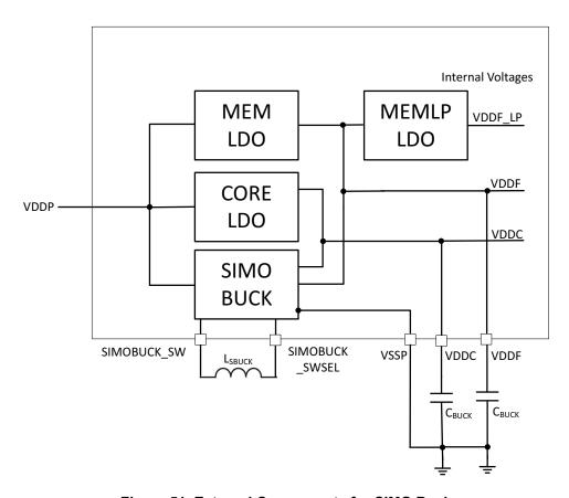
Figure 51. External Components for SIMO Buck
