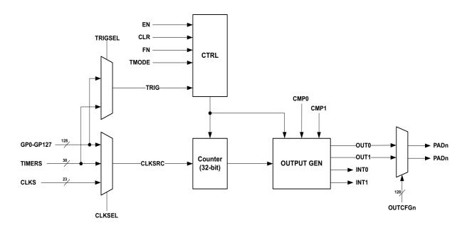
Figure 21. Block Diagram for One Counter/Timer
