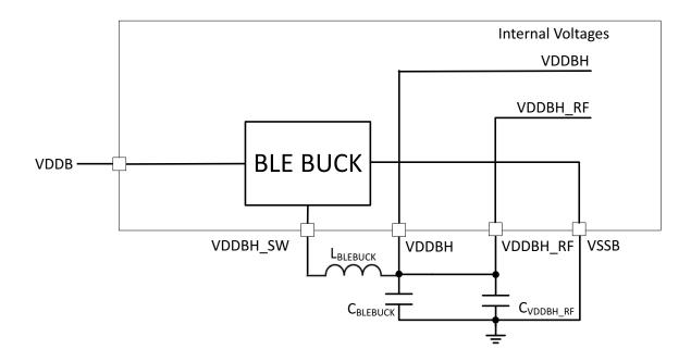
Figure 52. External Components for BLE Buck
