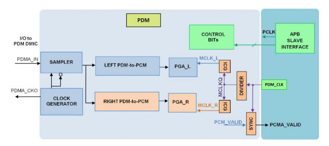
Figure 44. Clock Path and Data Synchronization Diagram
