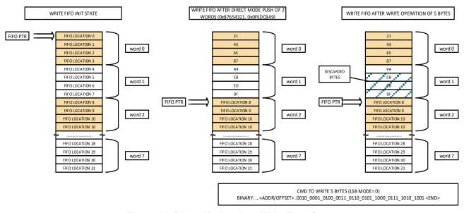
Figure 31. Direct Mode 5-byte Write Transfer
