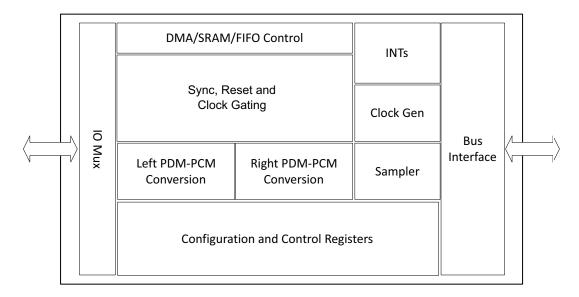
Figure 43. PDM Block Diagram
