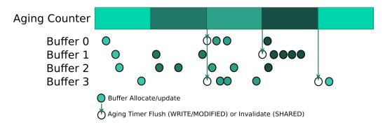
**Figure 6. Aging Counter Operation**
