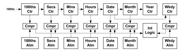
Figure 14. Block diagram for the Real Time Clock Module
