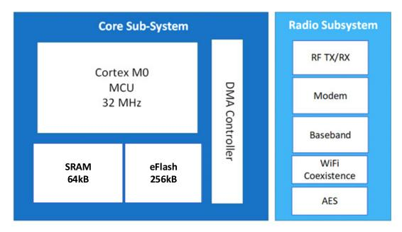
Figure 18. Apollo4 Blue Lite SoC Bluetooth Low Energy Controller Block Diagram
