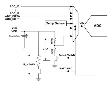
Figure 26. Switchable Battery Load
