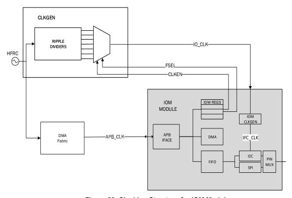
Figure 29. Clocking Structure for IOM Module
