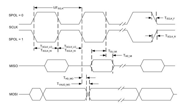
Figure 54. SPI Master Mode, Phase = 1
