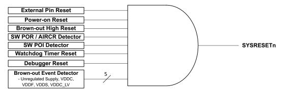
Figure 11. Block diagram for the Reset Generator Module
