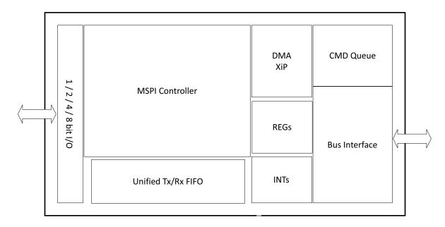
Figure 27. Block Diagram for the MSPI Master Module
