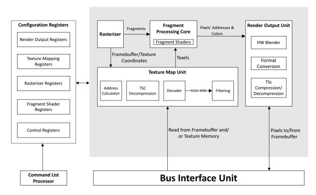
Figure 39. GPU Block Diagram
