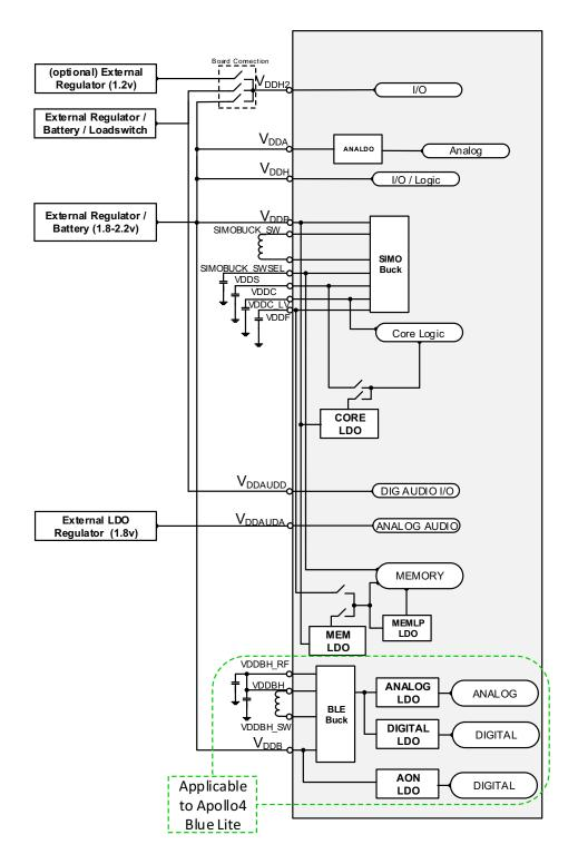
Figure 48. Block Diagram for Voltage Supplies and Regulation on Apollo4 Family
