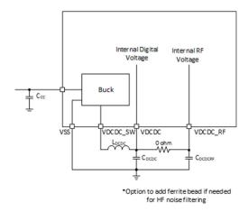
Figure 19. Integration Diagram for Buck Enabled Configuration
