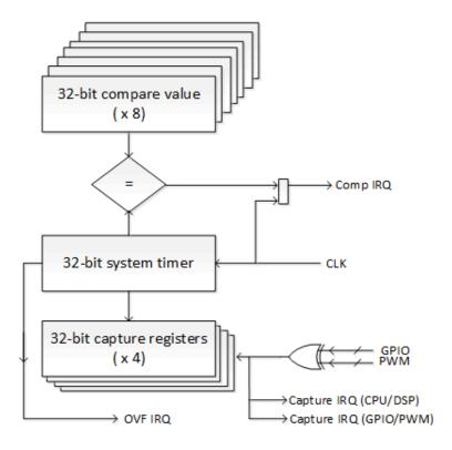
Figure 22. Block Diagram for the System Timer
