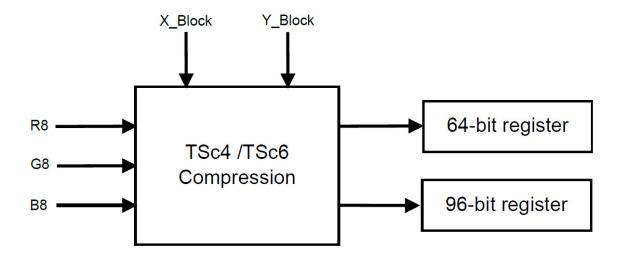
Figure 41. TSC™4 /TSC™6 Framebuffer Compression Module
