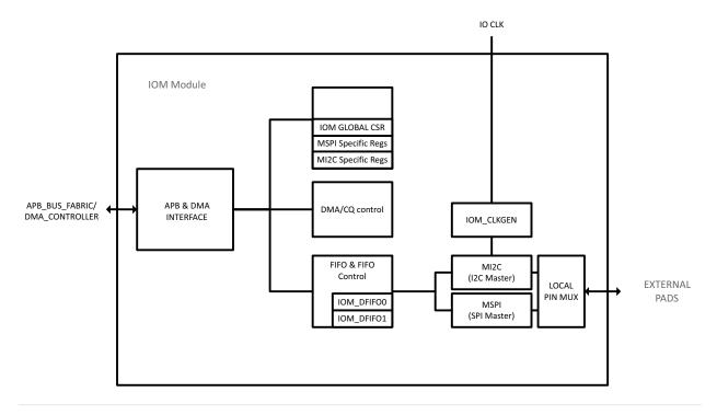
Figure 28. Block Diagram for the I<sup>2</sup>C/SPI Master Module
