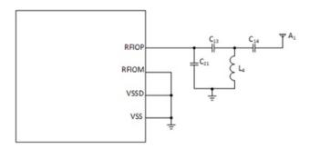
Figure 20. Recommended Antenna Filter
