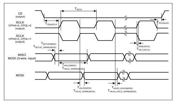
Figure 64. SPI Manager Interface Timing Diagram, CPHA = 0
