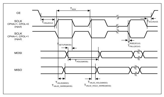
Figure 67. SPI Subordinate Interface Timing Diagram, CPHA = 1
