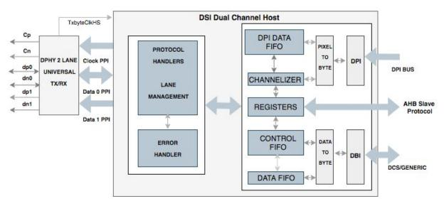
Figure 35. Block Diagram for the DSI Controller
