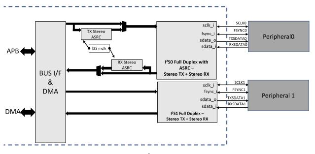
Figure 40. I<sup>2</sup>S Block Diagram
