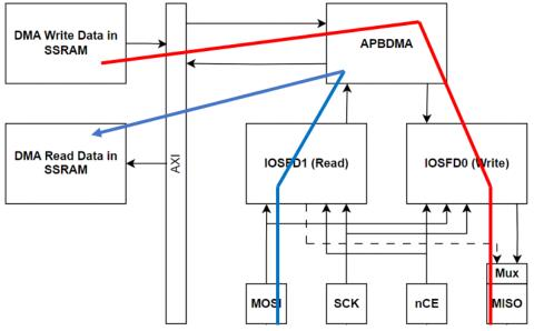
Figure 29. Full Duplex IOS DMA Transfers
