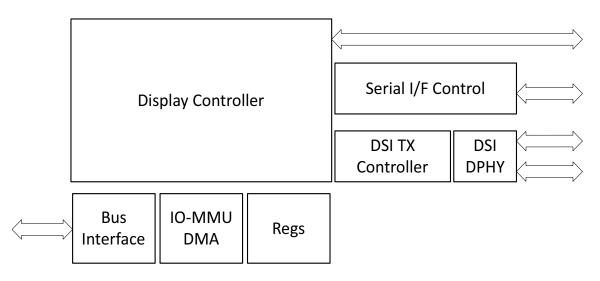
Figure 33. Block Diagram of the Display Subsystem
