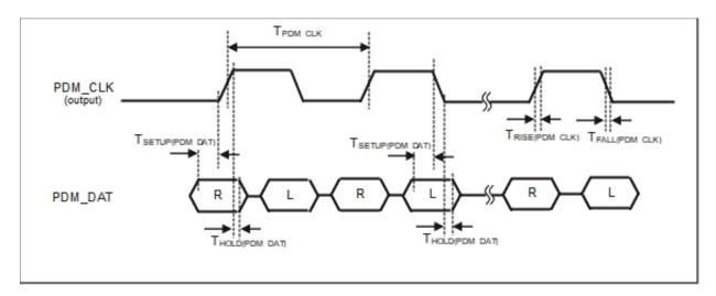
Figure 73. PDM Interface Timing Diagram
