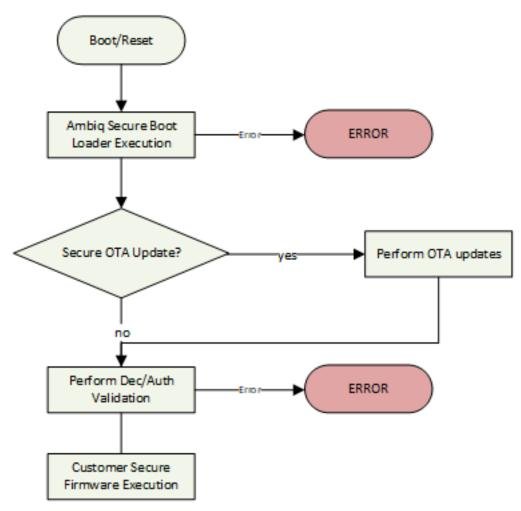
Figure 6. Secure Boot Process Flow Diagram
