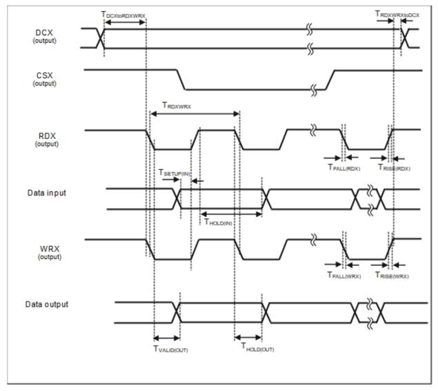
Figure 54. DC MIPI DBI-B Timing Diagram
