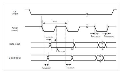
Figure 52. DC QSPI/SPI Timing Diagram
