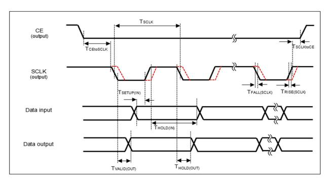
Figure 21. SDR Mode with Non-DQS
