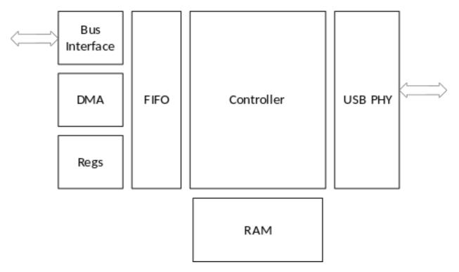
Figure 31. USB Block Diagram
