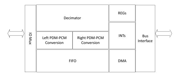
Figure 38. PDM Block Diagram
