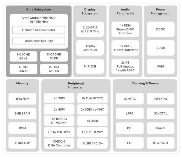
Figure 1. Apollo510 SoC High-Level Block Diagram
