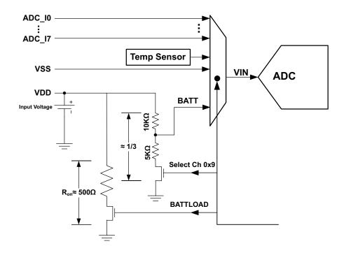
Figure 18. Switchable Battery Load
