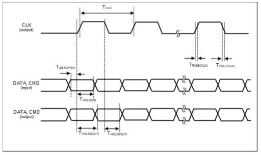
Figure 70. SD DDR50 Mode Interface Timing Diagram
