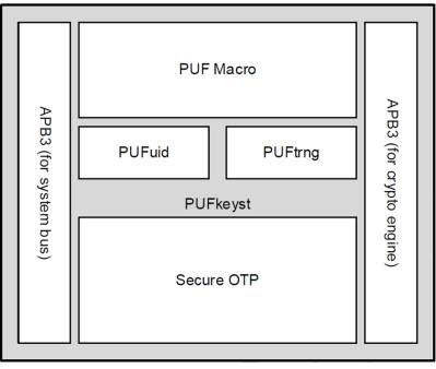
Figure 5. OTP Block Diagram
