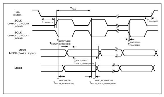
Figure 65. SPI Manager Interface Timing Diagram, CPHA = 1
