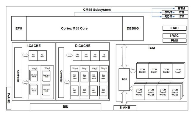
Figure 3. Apollo5 SoC Family CPU Subsystem Block Diagram
