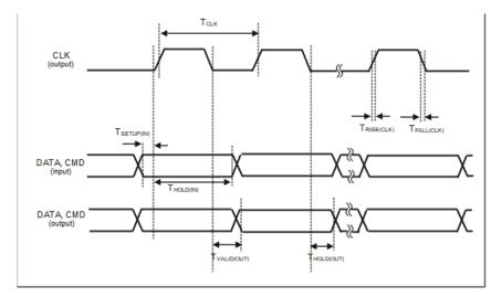
Figure 68. Default and High-Speed SD Interface Timing Diagram
