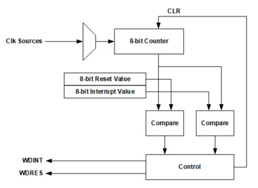
Figure 15. Watchdog Timer Block Diagram
