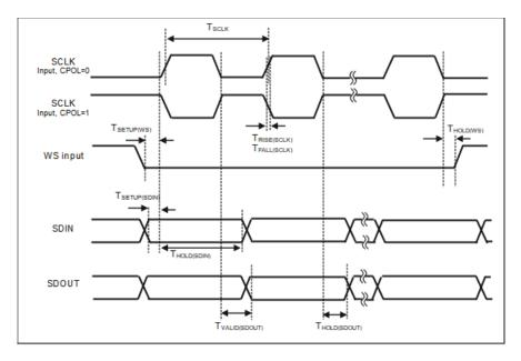
Figure 71. I<sup>2</sup>S Subordinate Interface Timing Diagram
