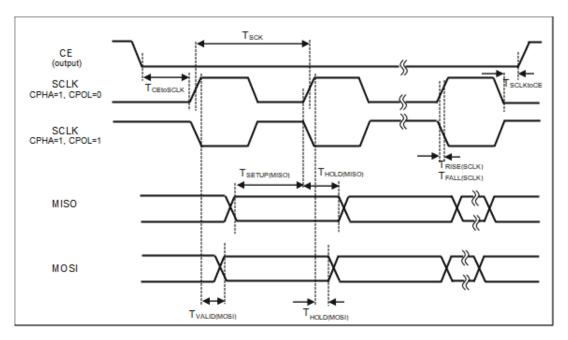
Figure 61. MSPI1/MSPI2 Standard 4-Wire Mode Timing Diagram - SPI Manager, CPHA=1
