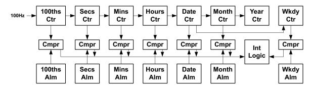
Figure 12. Block diagram for the Real Time Clock Module
