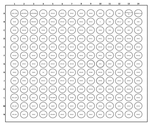
Figure 43. Apollo510 SoC WLCSP Pin Configuration Diagram - Top View
