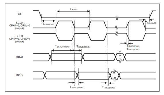
Figure 56. MSPI0/MSPI3 Standard 4-Wire Mode Timing Diagram - SPI Manager, CPHA=0
