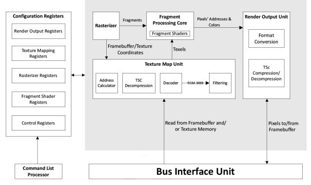
Figure 37. GPU Block Diagram
