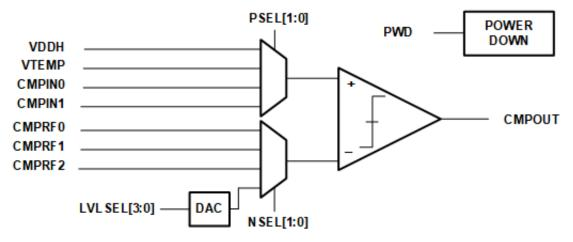
Figure 19. Voltage Comparator Block Diagram
