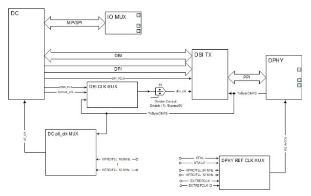
Figure 34. Display Controller Clocking Block Diagram
