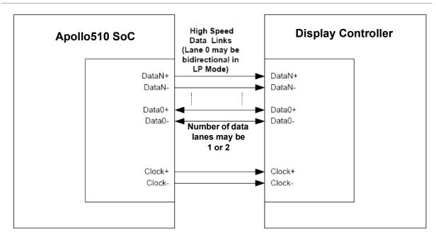
Figure 36. Display Serial Interface Bus with DSI Devices
