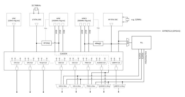
Figure 11. Block Diagram for Clock Generator Module
