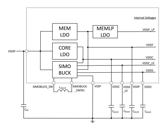
Figure 51. External Components for SIMO Buck
