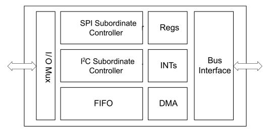
Figure 26. Block Diagram for IOS
