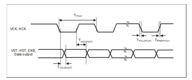
Figure 55. DC JDI MIP Timing Diagram
