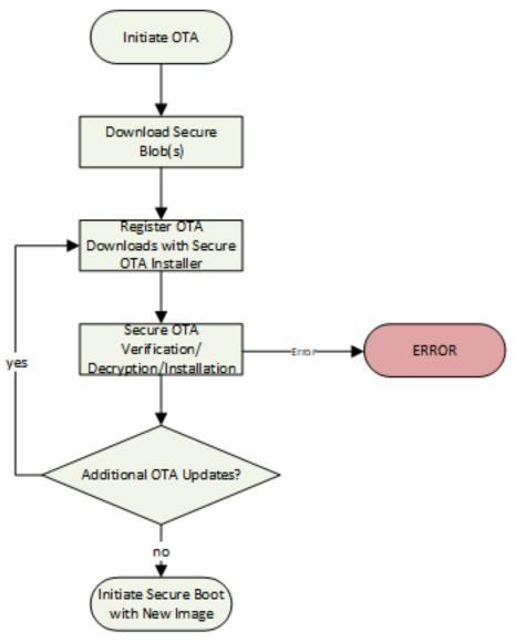
Figure 7. Secure OTA Flow Diagram
