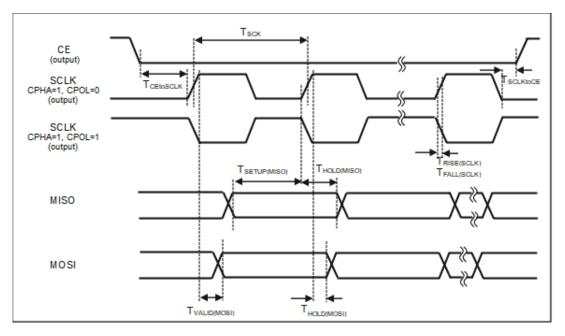
Figure 57. MSPI0/MSPI3 Standard 4-Wire Mode Timing Diagram - SPI Manager, CPHA=1
