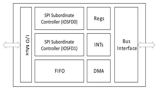
Figure 28. Full Duplex IOS SPI Subordinate Controller Pair (IOSFD0 / IOSFD1)
