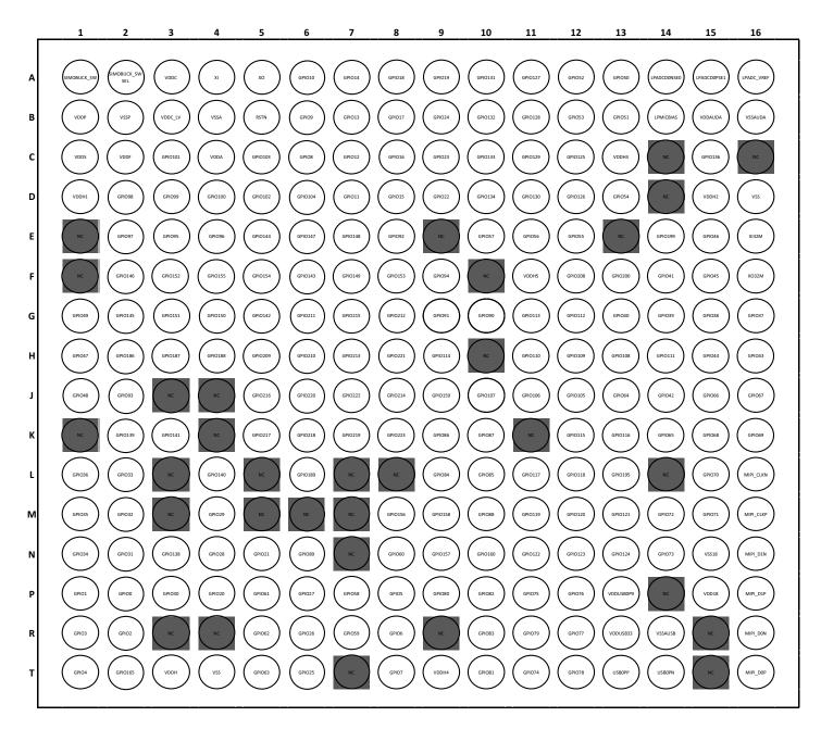
Figure 42. Apollo510 SoC BGA Pin Configuration Diagram - Top View
