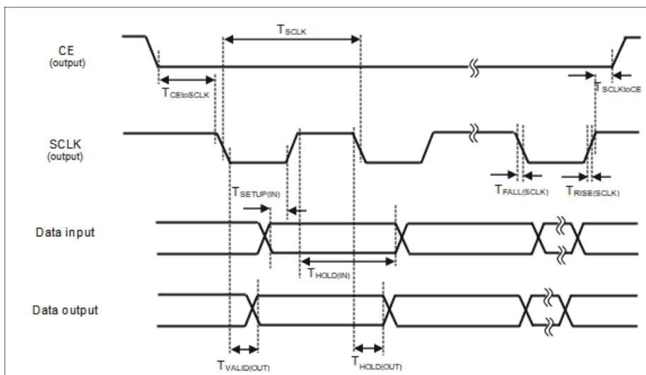
**Figure 62. MSPI1/MSPI2 SDR Non-DQS Mode Timing Diagram**
