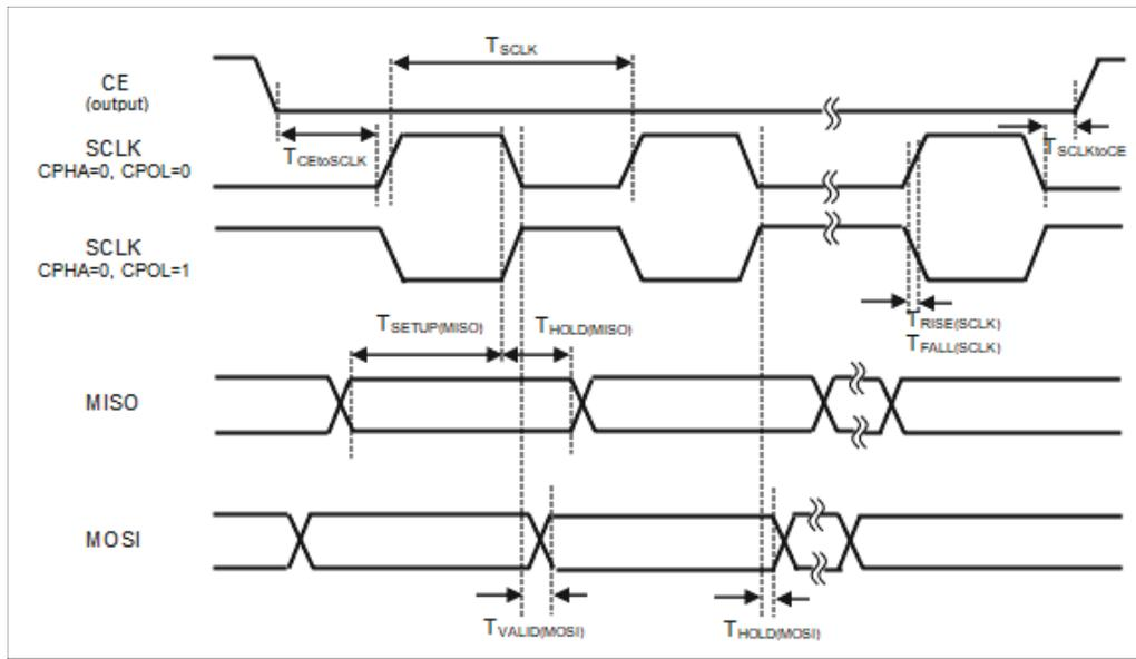
Figure 60. MSPI1/MSPI2 Standard 4-Wire Mode Timing Diagram - SPI Manager, CPHA=0
