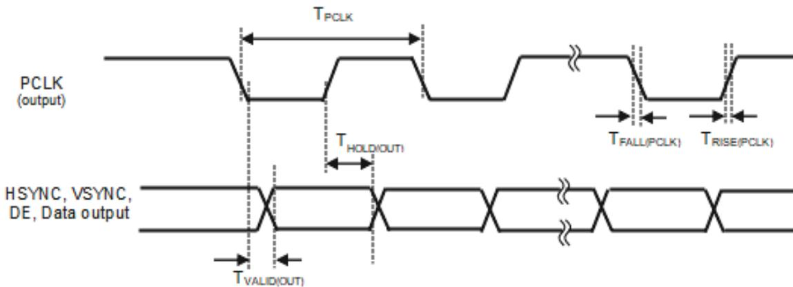
**Figure 53. DC MIPI DPI-2 Timing Diagram**
