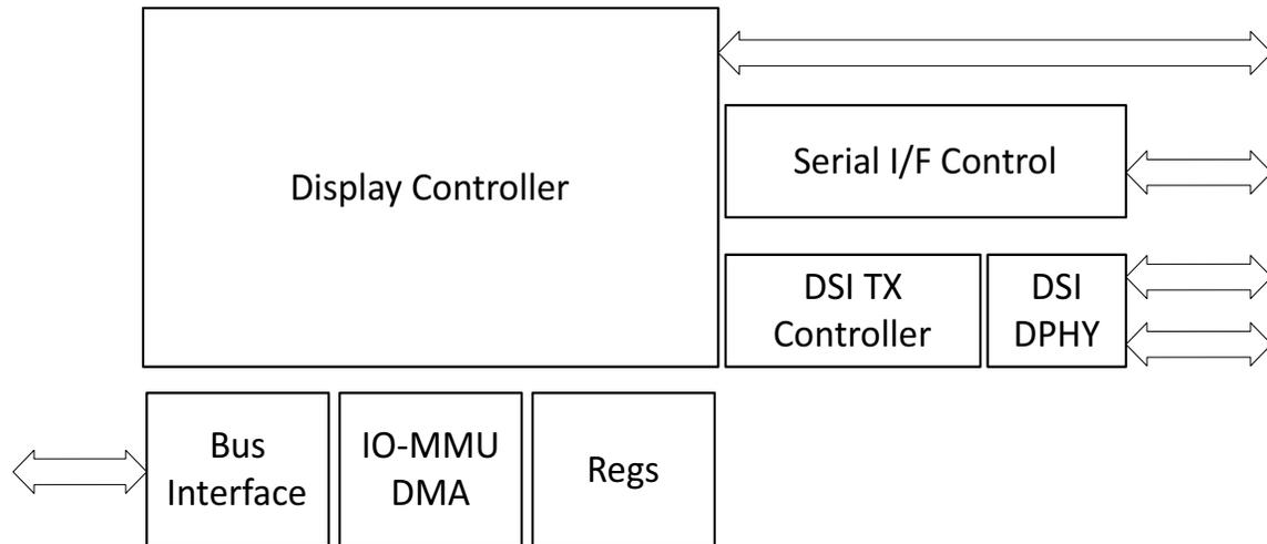
**Figure 33. Block Diagram of the Display Subsystem**
