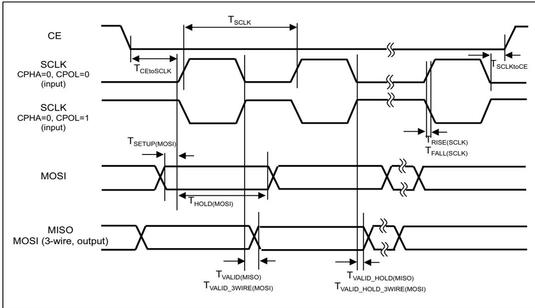
Figure 66. SPI Subordinate Interface Timing Diagram, CPHA = 0
