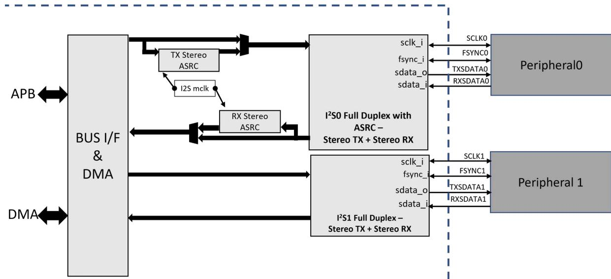
Figure 40. I<sup>2</sup>S Block Diagram
