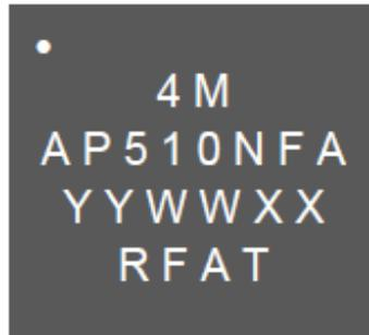
Figure 45. Apollo510 BGA Package Top Side Marking
