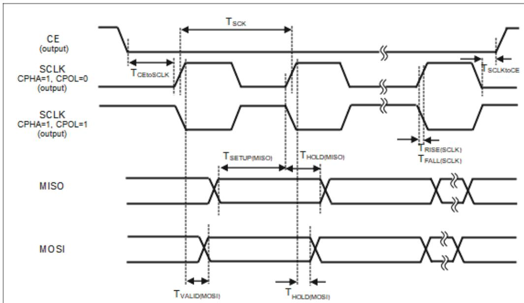
Figure 57. MSPI0/MSPI3 Standard 4-Wire Mode Timing Diagram - SPI Manager, CPHA=1
