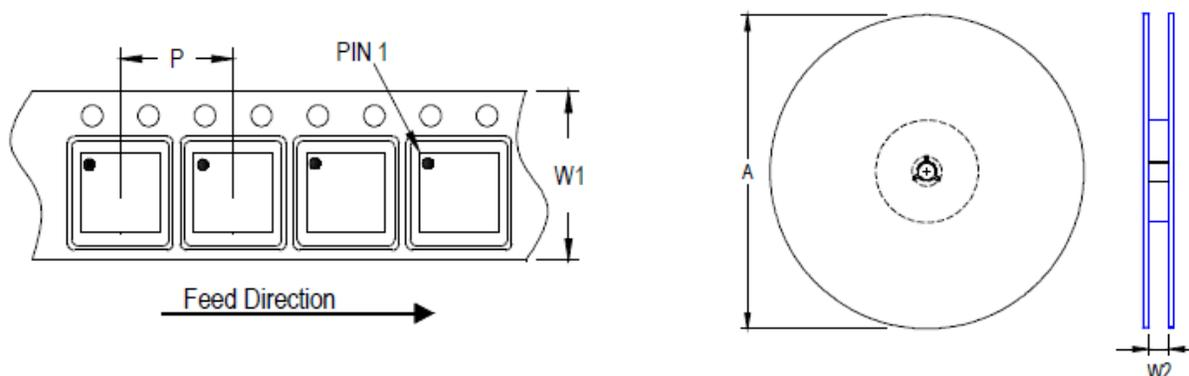
Figure 49. Tape Feed Direction and Reel Dimension Drawing
