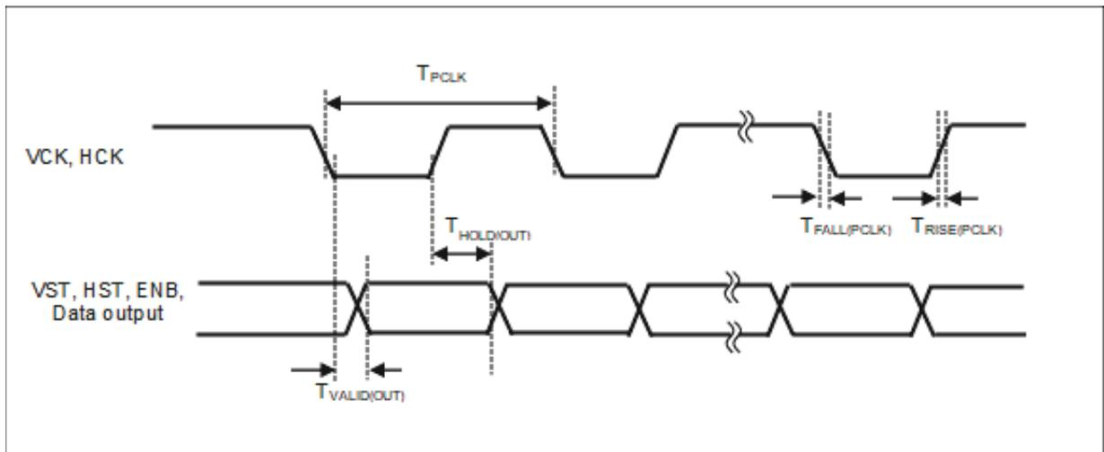
Figure 55. DC JDI MIP Timing Diagram
