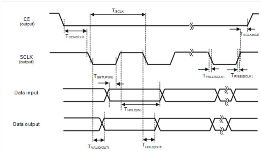
Figure 58. Timing Diagram for MSPI0/MSPI3 SDR Non-DQS Mode
