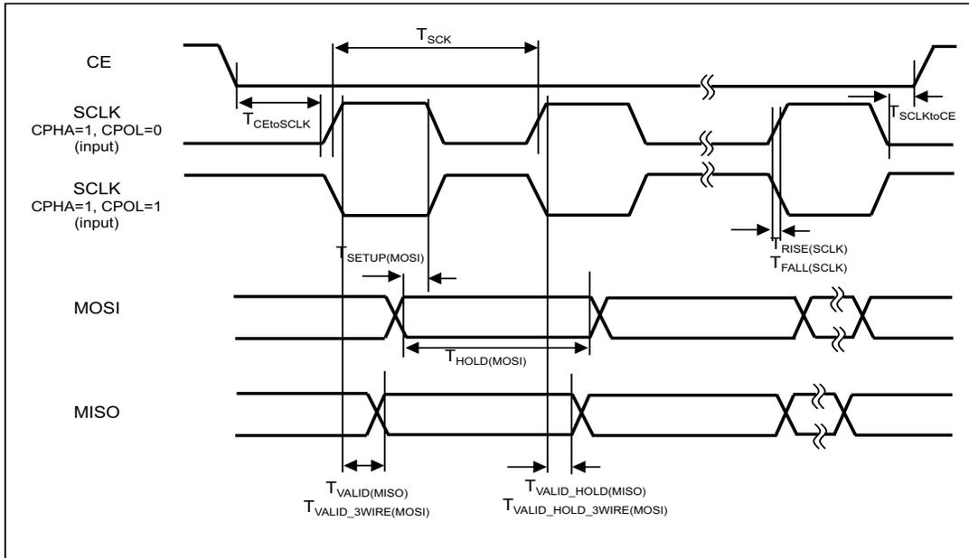
Figure 67. SPI Subordinate Interface Timing Diagram, CPHA = 1
