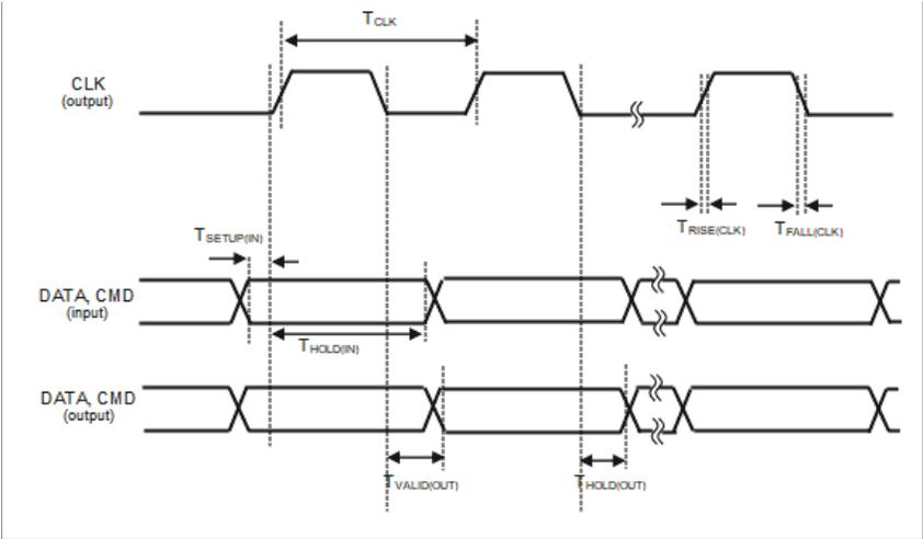
Figure 68. Default and High-Speed SD Interface Timing Diagram
