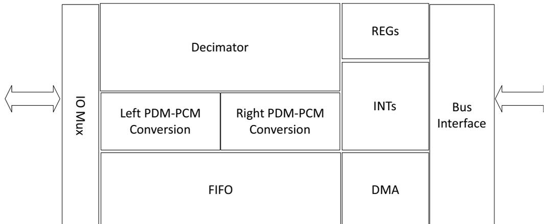
Figure 38. PDM Block Diagram
