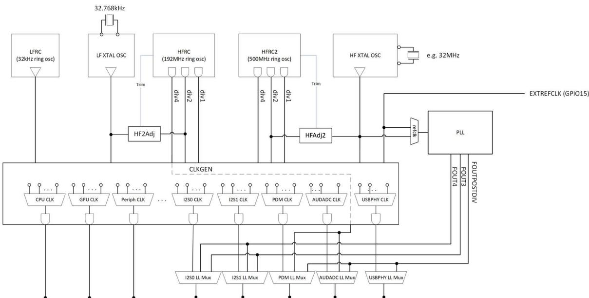
Figure 11. Block Diagram for Clock Generator Module
