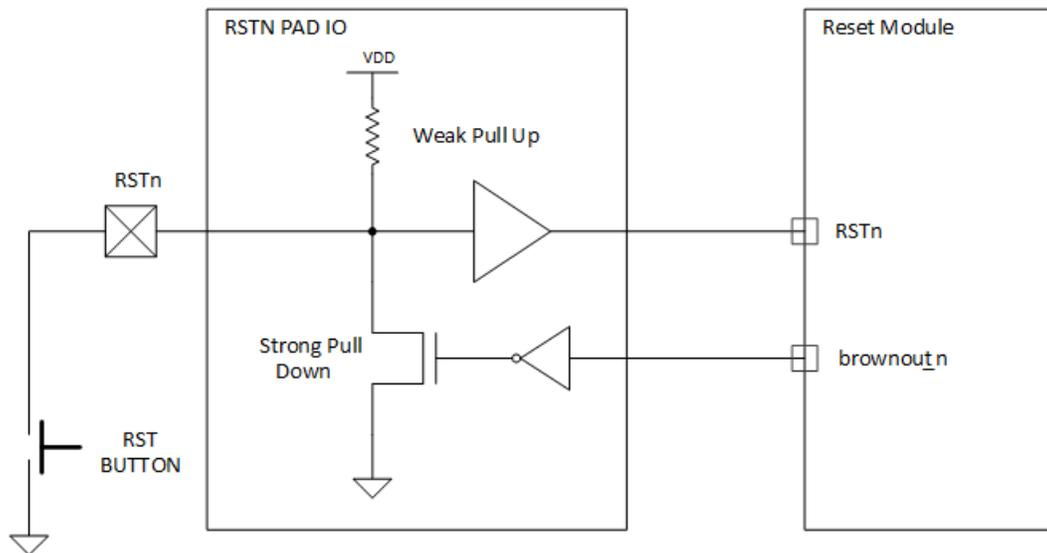
**Figure 10. Block Diagram of Reset Pin Circuitry**
