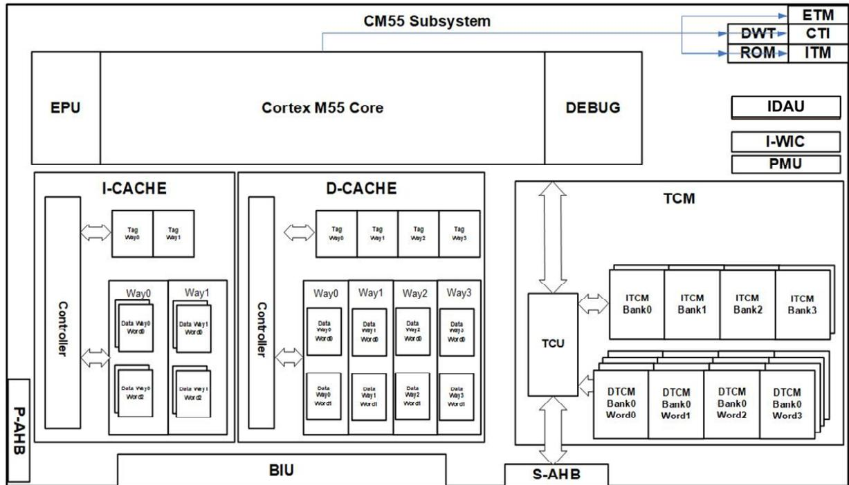
Figure 3. Apollo5 SoC Family CPU Subsystem Block Diagram
