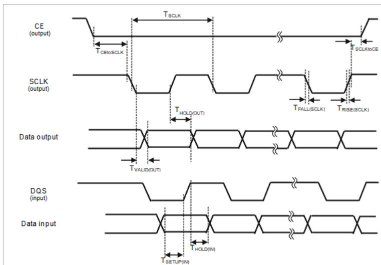
Figure 59. MSPI0/MSPI3 DDR with DQS Mode Timing Diagram
