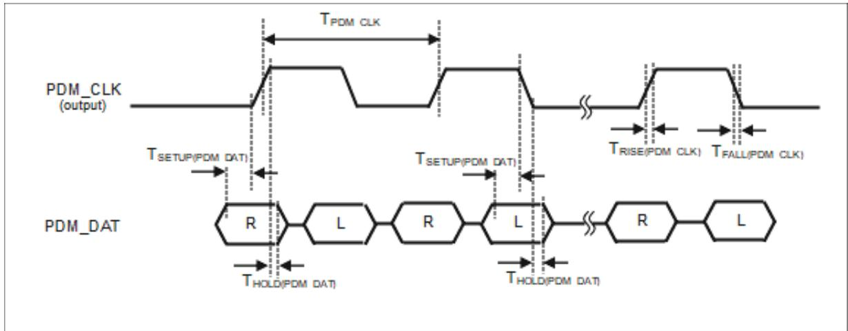
Figure 73. PDM Interface Timing Diagram
