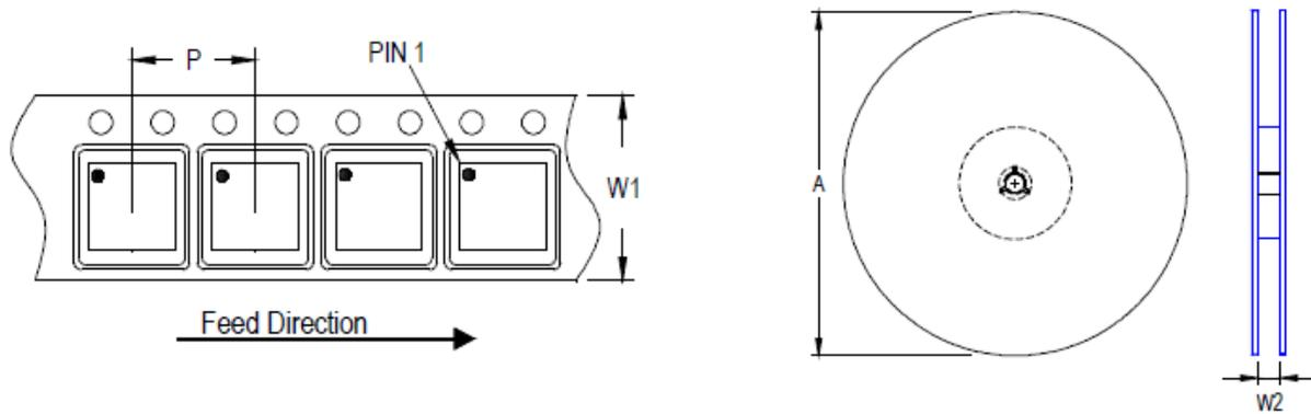
Figure 46. Tape Feed Direction and Reel Dimension Drawing
