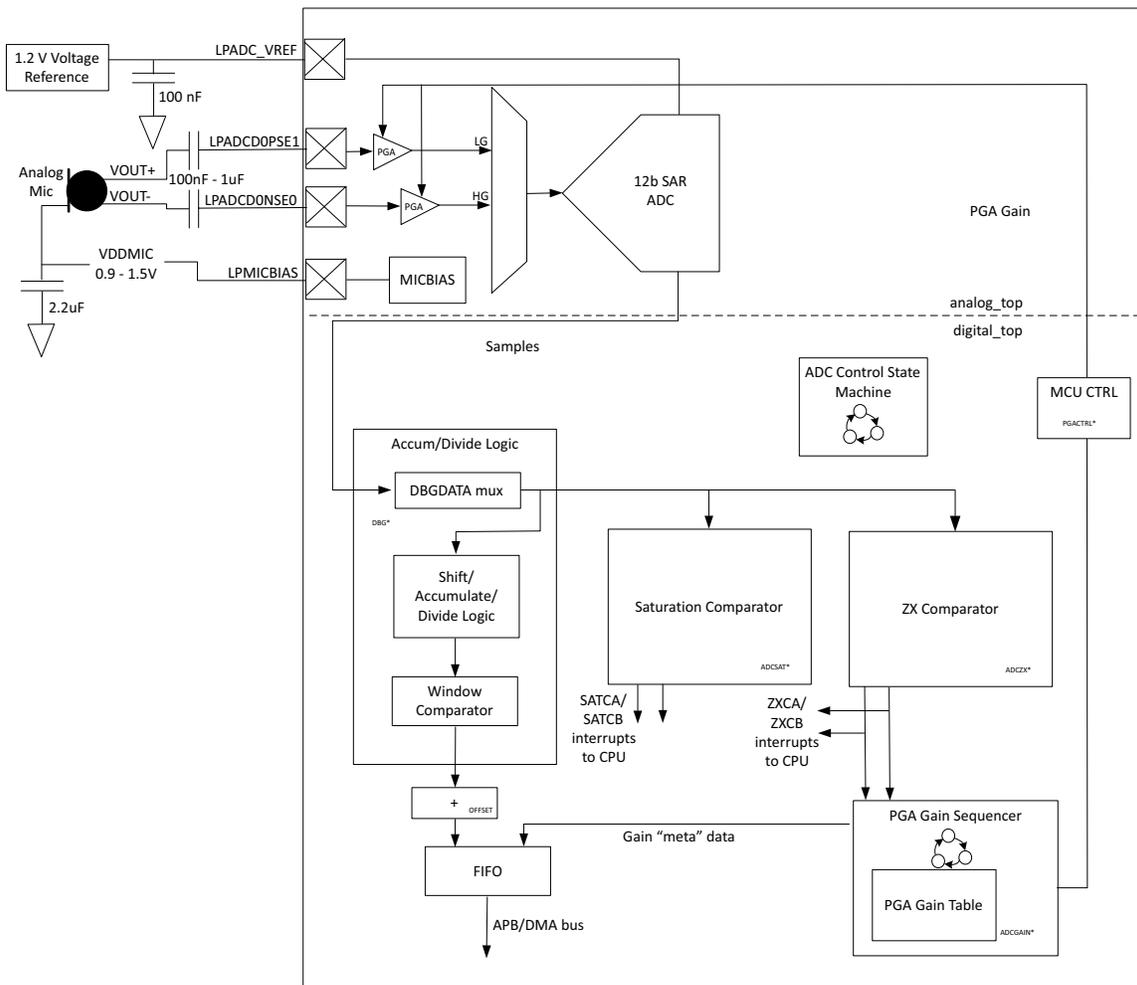
Figure 39. Low Power Analog Audio Interface Block Diagram
