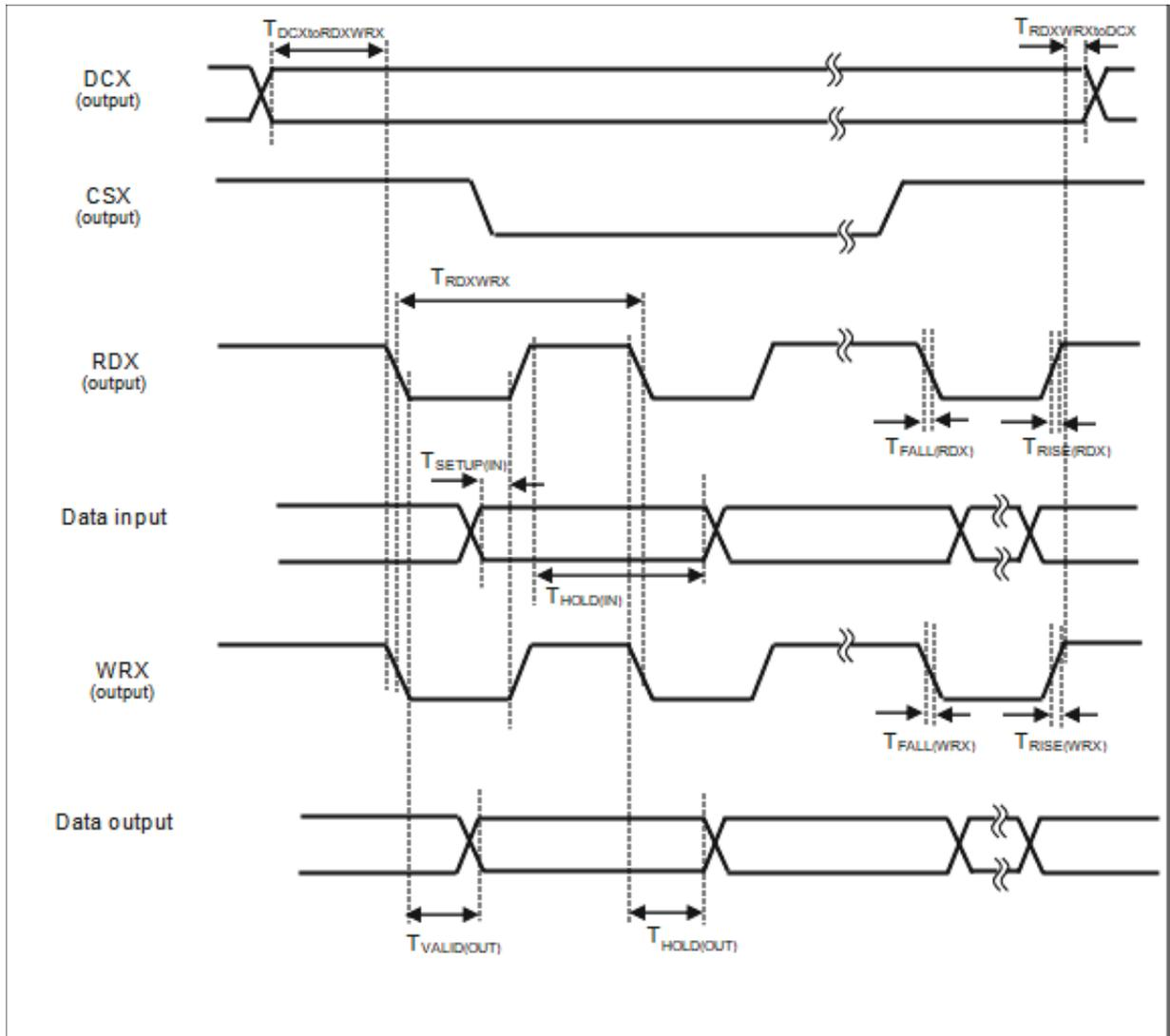
Figure 54. DC MIPI DBI-B Timing Diagram
