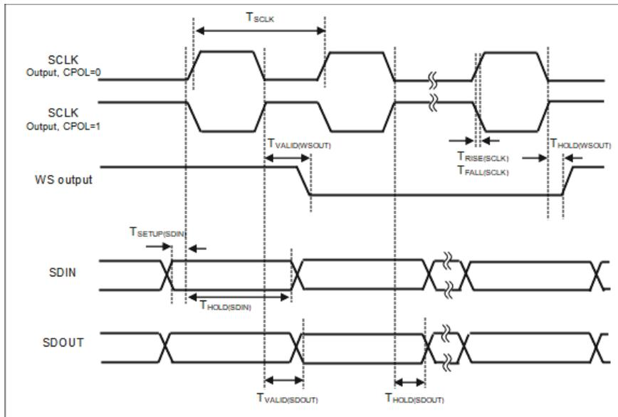
**Figure 72. I<sup>2</sup>S Manager Interface Timing Diagram**
