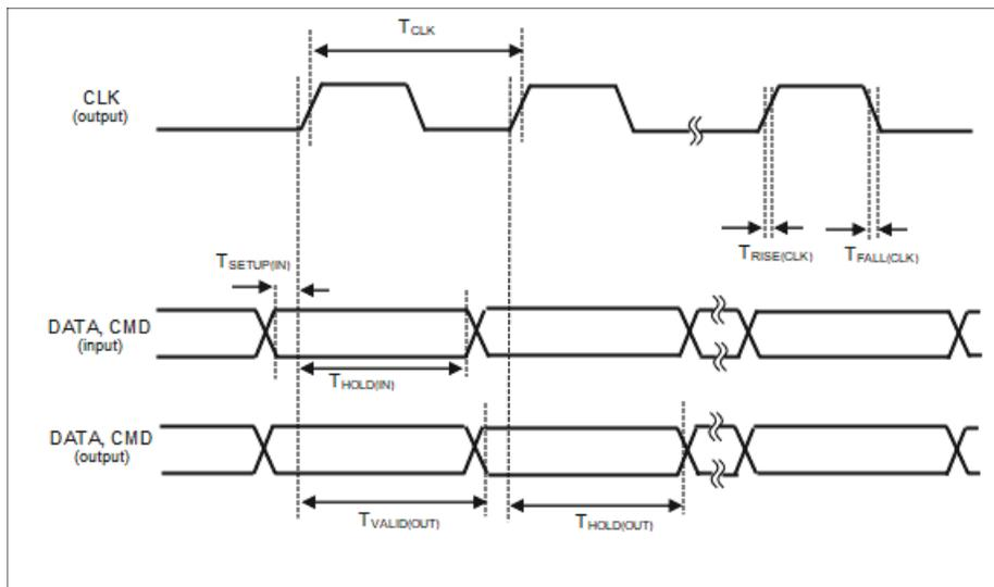
**Figure 69. SD SDR50 Mode Interface Timing Diagram**
