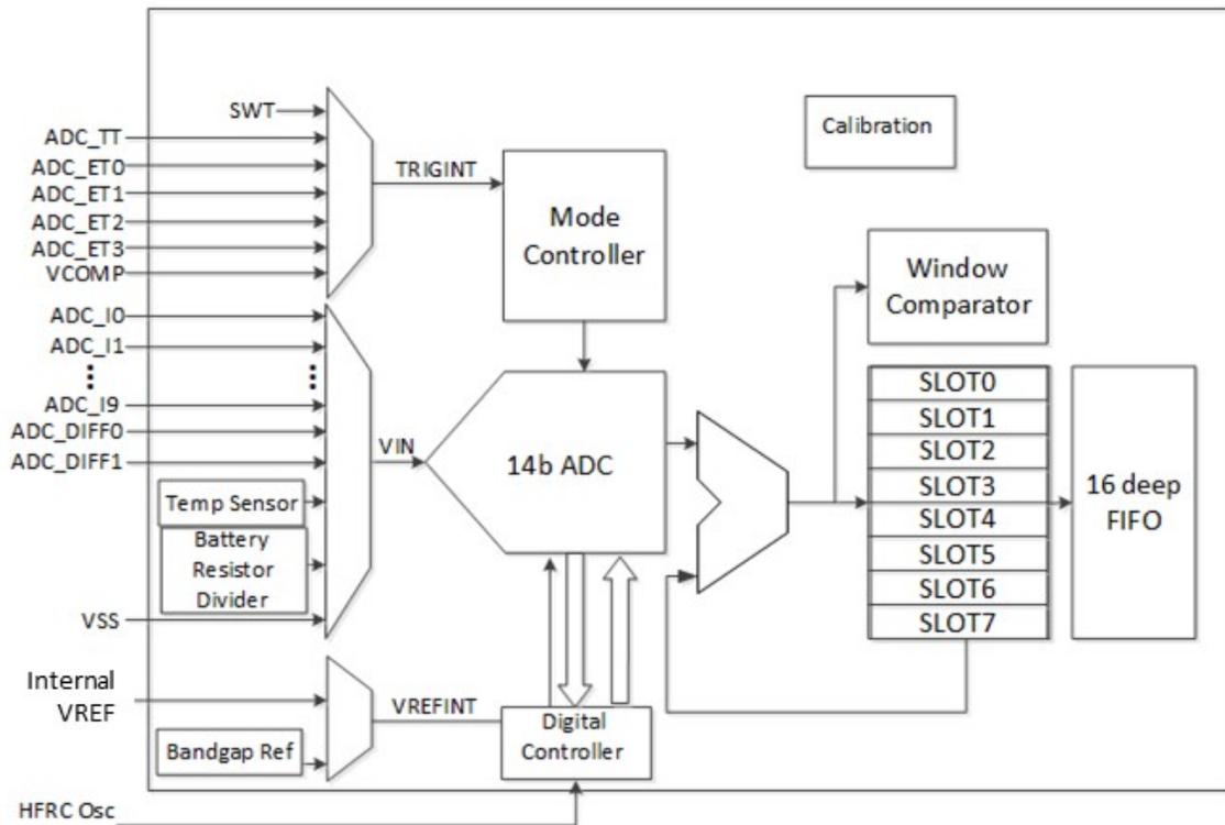
Figure 17. Block Diagram for ADC and Temperature Sensor
