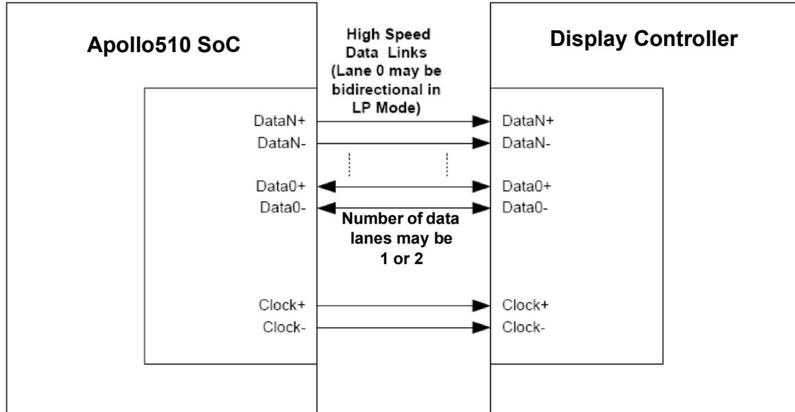
**Figure 36. Display Serial Interface Bus with DSI Devices**
