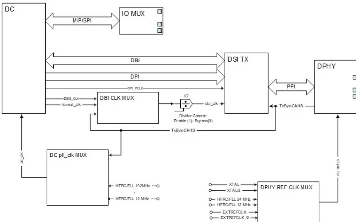
Figure 34. Display Controller Clocking Block Diagram
