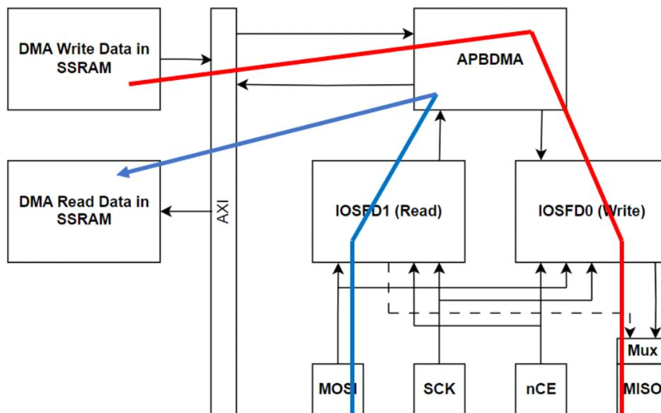
Figure 29. Full Duplex IOS DMA Transfers
