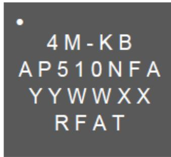
Figure 48. Apollo510 WLCSP Top Side Marking
