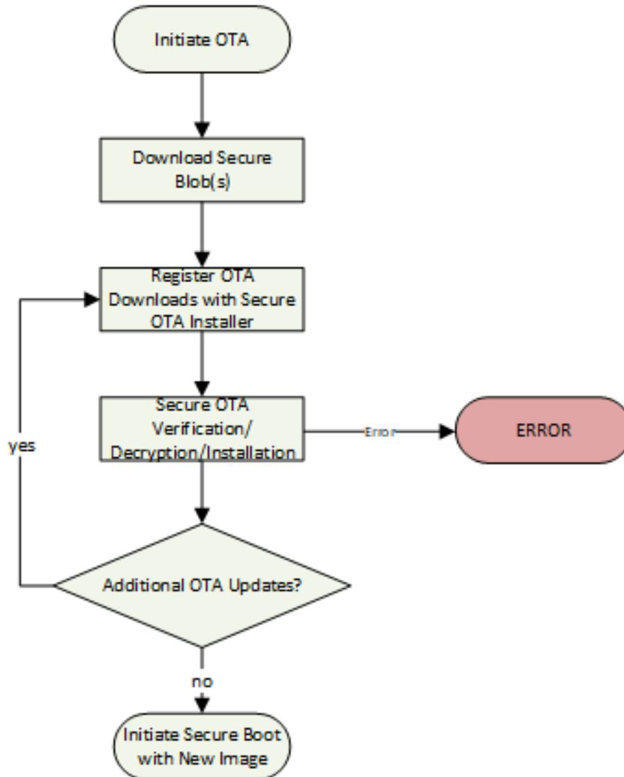
Figure 7. Secure OTA Flow Diagram
