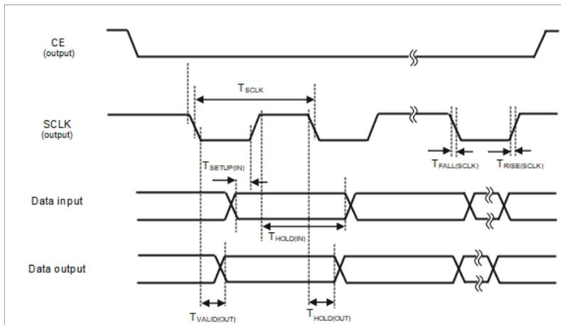
Figure 52. DC QSPI/SPI Timing Diagram
