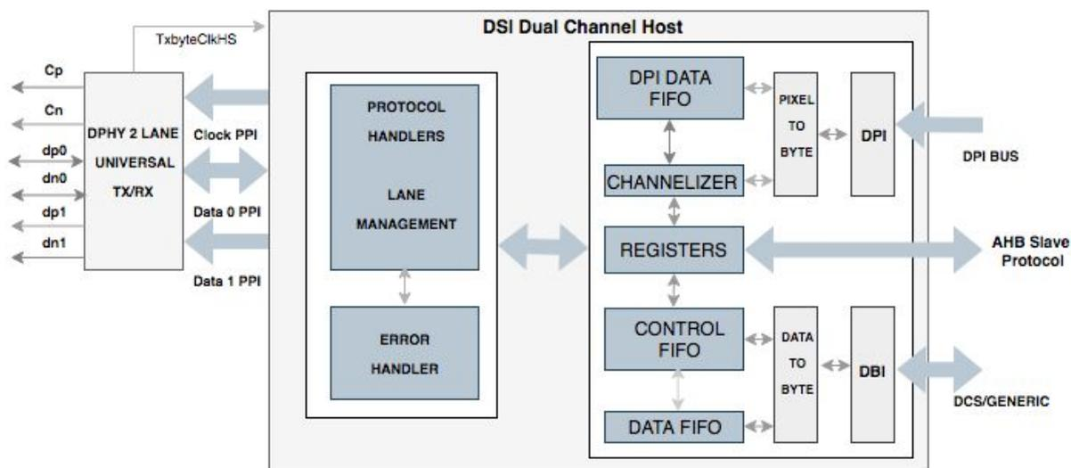
Figure 35. Block Diagram for the DSI Controller
