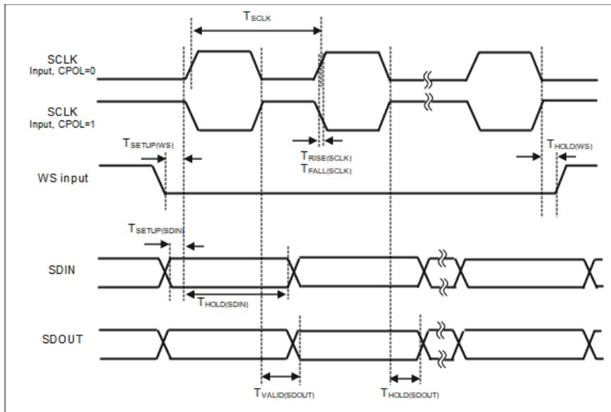
Figure 71. I<sup>2</sup>S Subordinate Interface Timing Diagram
