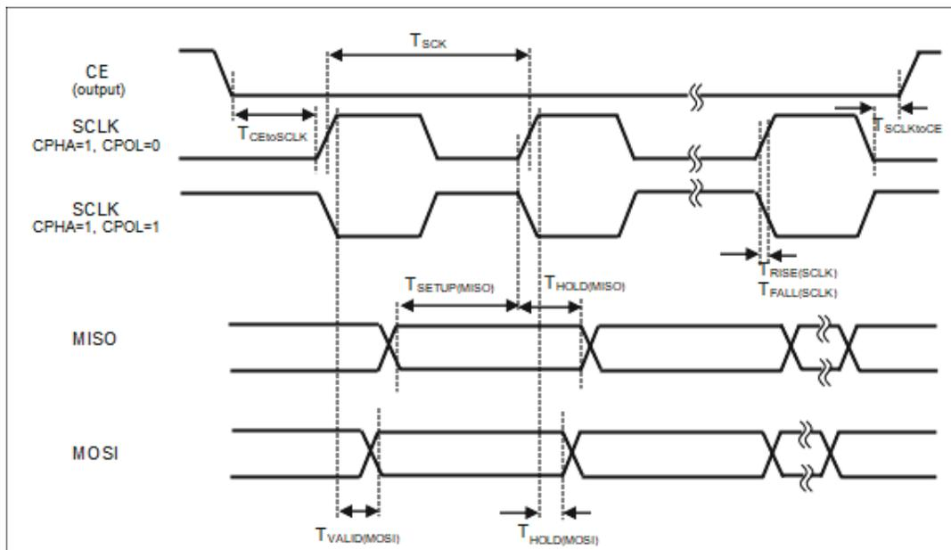
Figure 61. MSPI1/MSPI2 Standard 4-Wire Mode Timing Diagram - SPI Manager, CPHA=1
