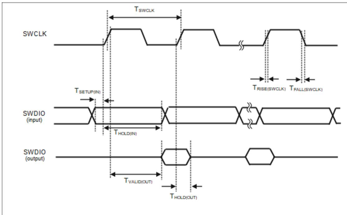
Figure 74. SWD Interface Timing Diagram
