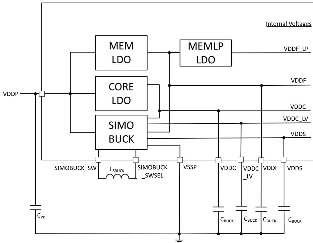
Figure 51. External Components for SIMO Buck
