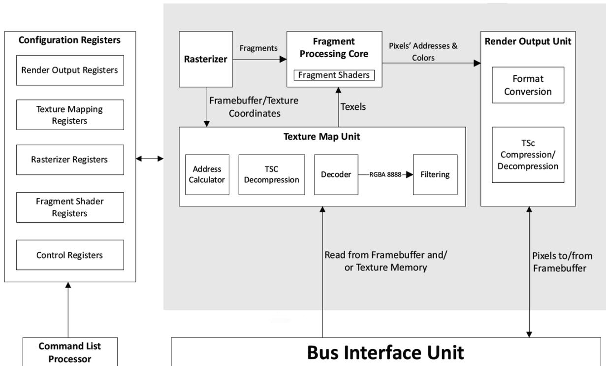
Figure 37. GPU Block Diagram
