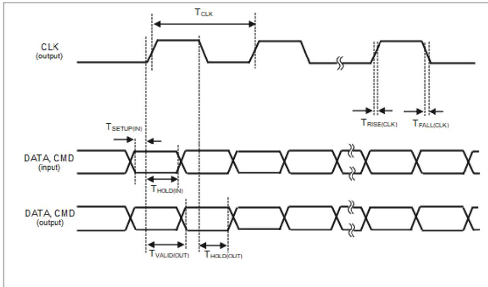
**Figure 70. SD DDR50 Mode Interface Timing Diagram**
