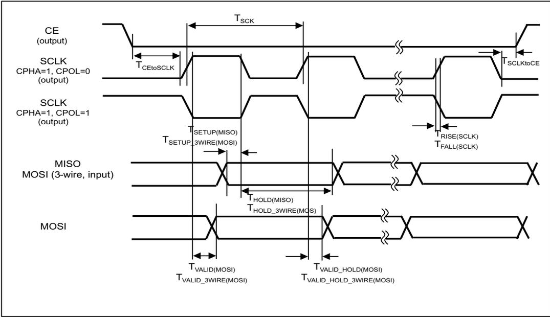
Figure 65. SPI Manager Interface Timing Diagram, CPHA = 1
