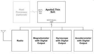
Typical Sensor Application Circuit for the Apollo2 Thin SoC
