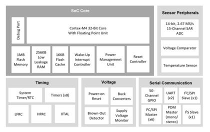
Block Diagram for the Ultra-Low Power Apollo2 Thin SoC
