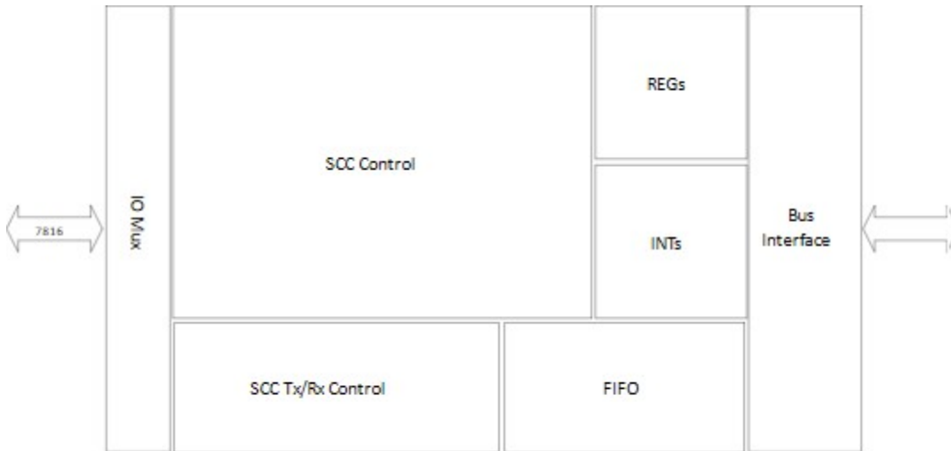
Figure 89. Block Diagram for the Secure Card Module
