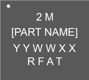
Figure 51. Apollo330 Plus Series SoCs BGA Package Top Side Marking
