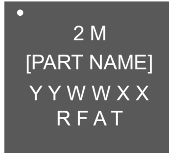
Figure 58. Apollo510 Lite Series SoCs BGA Package Top Side Marking
